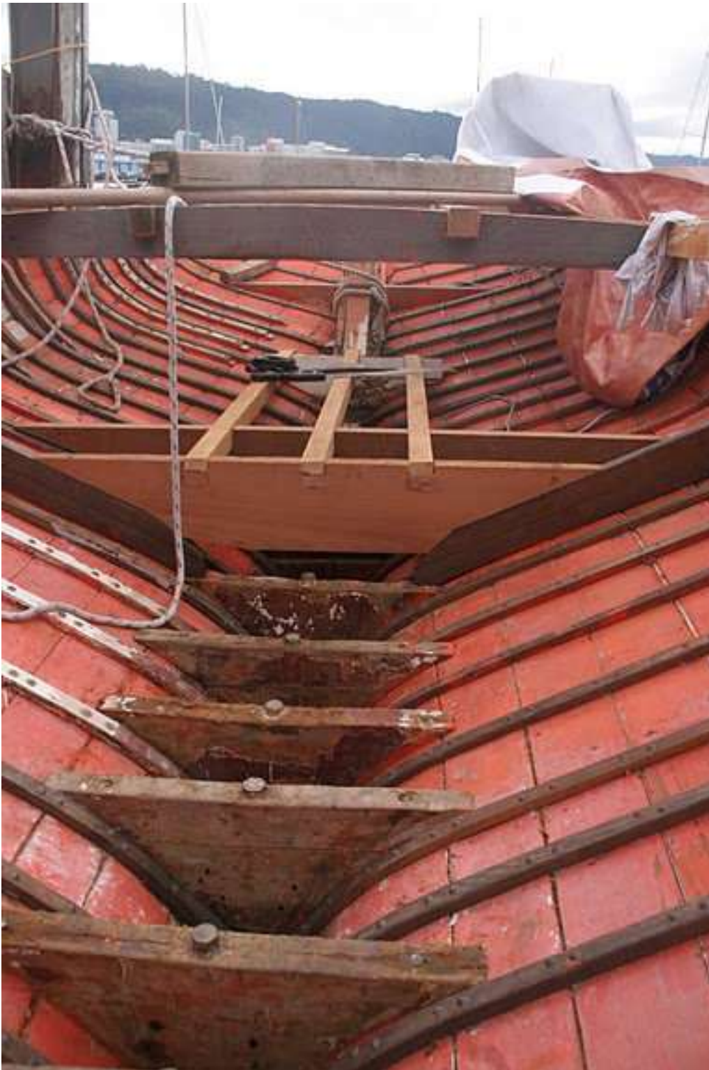
Reframing nearing completion 2011
